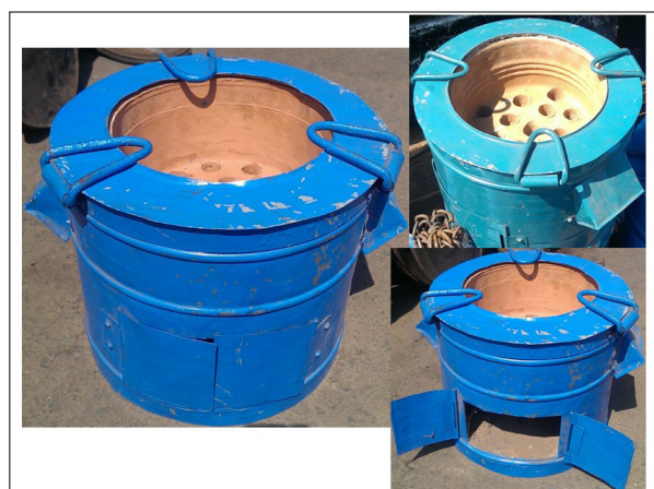
Figure 3. The Uga Cookstove: uses charcoal, locally made in Uganda (credit Gasim Omer Elkhaila Abd-Elfarag)
