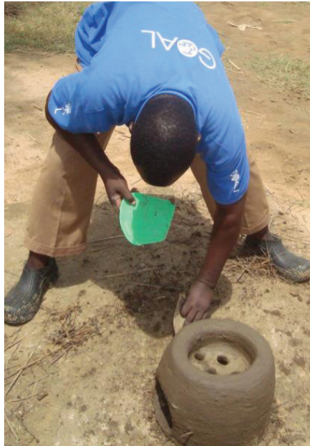
Figure 1. Construction of Fuel-Efficient Stoves – training in Twic County, Warrap State (credit Frank Okello)
