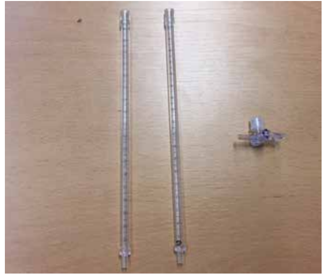
Figure 5. Manometer with three way tap (stopcock) used for the measurement of opening and closing pressures
