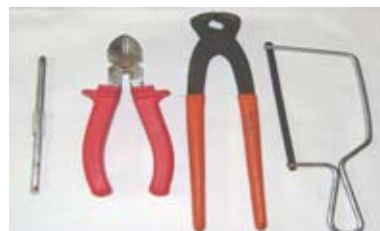
Figure 2. Technician's instruments for removing objects stuck on fingers (from left to right: screw driver without a handle, wire strippers, wire cutters and a junior hack saw).
